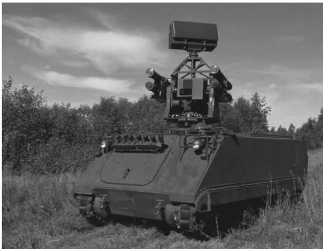
**Fig. 6:** The ASRAD-R with Bolid missile and the HARD 3D search radar
