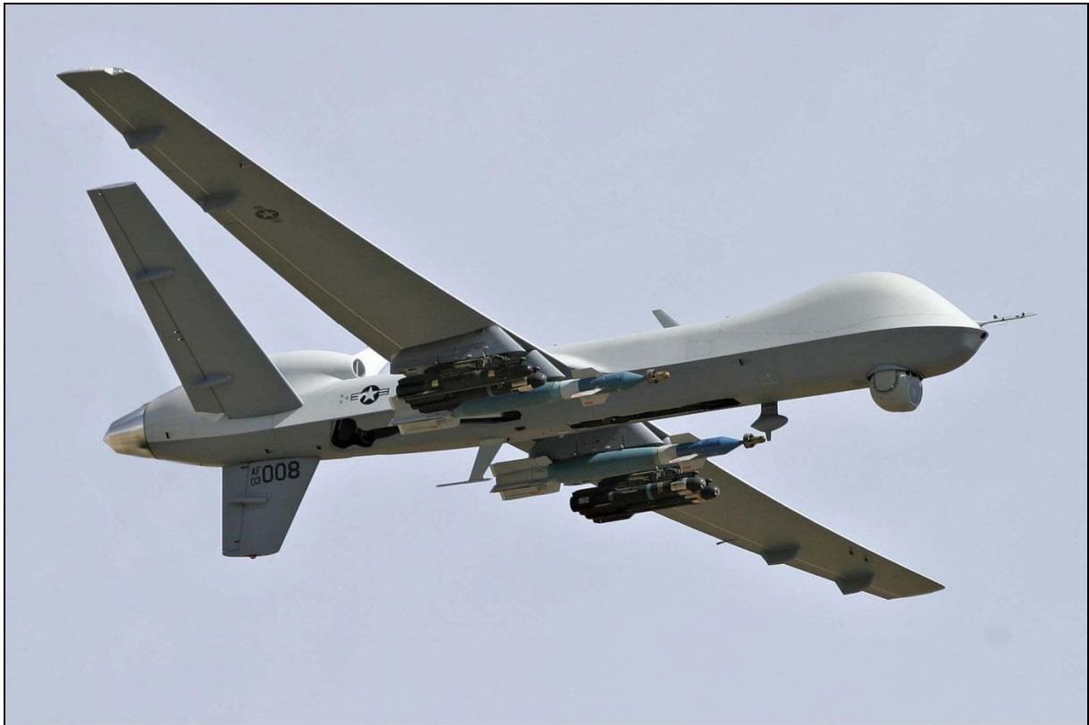
Figure 1. Remote Piloted Air System (RPAS) MQ-1 Predator, used by the American military. Predator's payload consists of four or eight Hellfire Missiles AGM-114C or AGM-176B Griffin (INS / GPS + semi-active laser guidance) with a weight of approximately 15 kg with a range of 8 to 20 km; and two Paveway II laser guided bombs GBU-39B, GBU-58 or GBU-44/B Viper Strike. Adopted from: "Amerykańskie Reapery w bazie w Mirosławcu". Radar rp.pl, by Z. Lewitowicz, Copyright 2019 by the Publisher. https://radar.rp.pl/wojsko-polskie/13633-amerykanskie-reapery-w-bazie-w-miroslawcu
