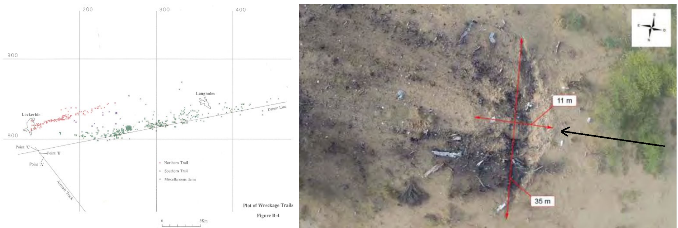
Figure 2. A comparison of aircraft remains scattering without an explosion and after an explosion.
