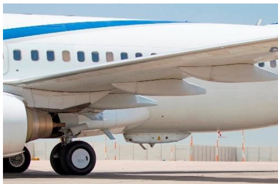
Figure 1. El Al’s Boeing 757-800 equipped with C-MUSIC system. Adopted from: (Altair, 2014).
